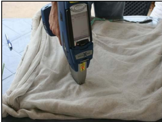
Figure 3. X-ray fluorescence to measure deltamethrin.
